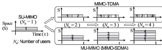
Fig. 12 Resource allocations for MIMO-TDMA and MU-MIMO.
