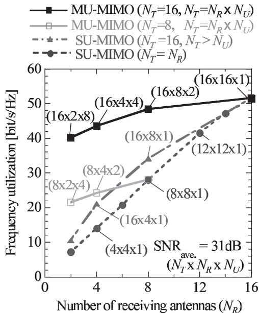
Fig. 10 Frequency utilization comparison between MU-MIMO and SU-MIMO.
