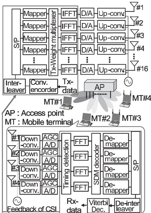
Fig. 1 Block diagram of 16 × 16 MU-MIMO testbed.
