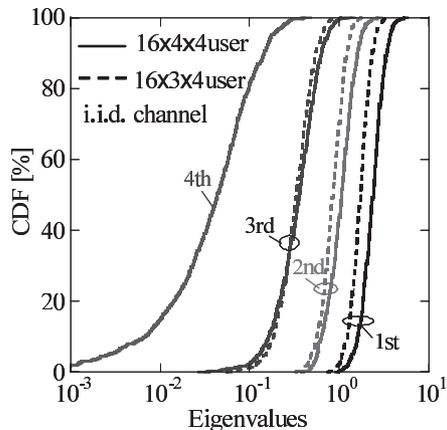
Fig. 4 Eigenvalue distribution when using BD algorithm.
