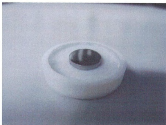
(a) Disk specimen installed on the water cell
