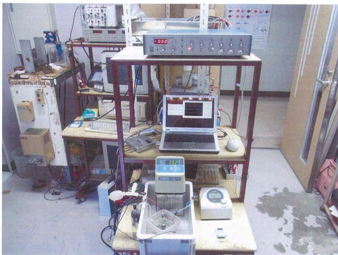
Fig. 5.2.6 Measuring system for electrical polarization test
