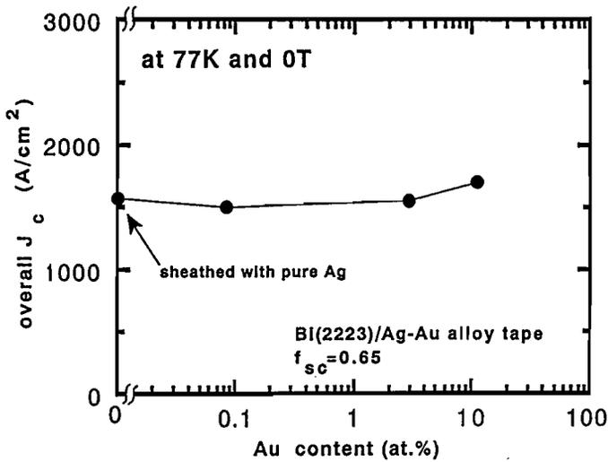
Fig. 7. Overall- $J_c$  of the Bi-2223 superconducting tapes with various concentrations of Au at 77K and 0T, in which the superconducting core ratio  $f_{sc}$  is 0.65.
