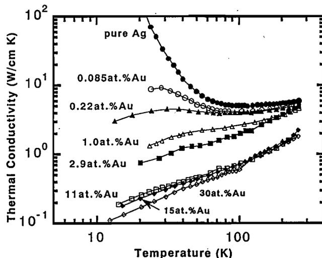
Fig. 1. Temperature dependence of the thermal conductivity of heat treated Ag-Au alloy tapes with the various concentrations of Au.
