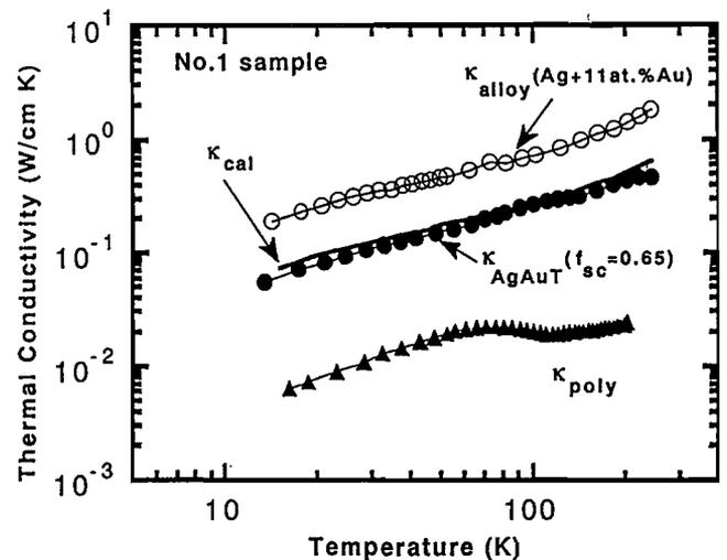
Fig. 4. Temperature dependence of the thermal conductivity  $\kappa_{AgAuT}$  of Bi-2223 superconducting tape (No.1 sample) sheathed with Ag+11at.%Au alloy for ratio  $f_{sc}$  0.65 (closed circles). The thermal conductivity of Ag+11at.%Au alloy tape  $\kappa_{alloy}$  (open circles) and that of Bi-2223 polycrystal  $\kappa_{poly}$  (closed triangles) and the calculated thermal conductivity  $\kappa_{cal}$  (thick line) were also shown.
