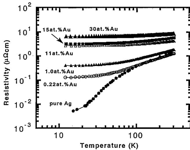
Fig. 2. Temperature dependence of the electrical resistivity of heat treated Ag-Au alloy tapes with the various concentrations of Au.
