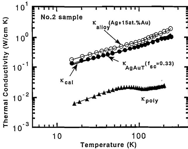
Fig. 5. Temperature dependence of the thermal conductivity of Bi-2223 superconducting tape (No.2 sample) sheathed with Ag+15at.%Au alloy for core ratio  $f_{sc}$  0.33 (closed circles). The thermal conductivity of Ag+15at.%Au alloy tape (open circles), that of Bi-2223 polycrystal (closed triangles) and the calculated thermal conductivity (thick line) are also shown.
