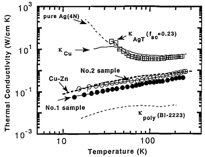
Fig. 6. Temperature dependence of thermal conductivities of both the Bi-2223 superconducting tapes sheathed with pure Ag ( $f_{sc} = 0.23$ ) and the high purity copper of 4N grade. For comparison, the thermal conductivities of the pure Ag(4N) tape, No.1 and 2 samples, a Cu-Zn alloy and Bi-2223 polycrystal are also shown.
