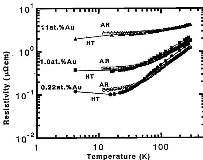
Fig. 3. Temperature dependence of the electrical resistivities of both the as-rolled Ag-Au tapes (AR) and the heat treated tapes (HT) in which Au contains from 0.22 to 11at.%.
