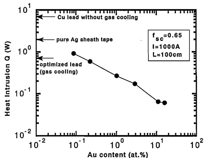
Fig.9. Relation between the heat intrusion through a 100cm superconducting lead of 1000A which is  $f_{sc}=0.65$  and the Au content in the Ag-Au alloy sheath.
