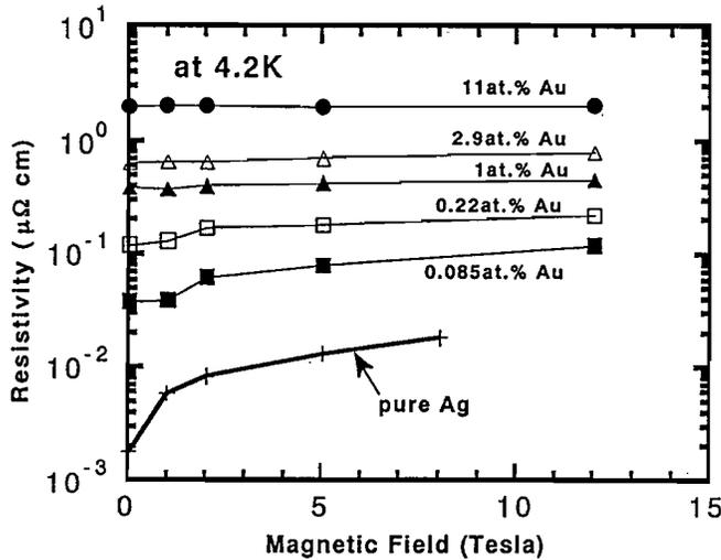
Fig. 10. Magnetic field dependence of the electrical resistivity of Ag-Au alloys with various concentrations of Au at 4.2K.
