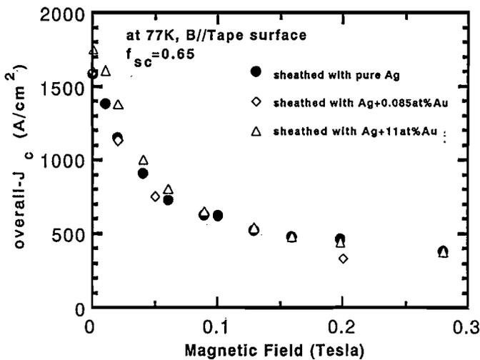
Fig. 8. Overall- $J_c$  vs. applied magnetic field curves with various Au contents in the Ag-Au alloy sheathes at 77K. The magnetic field was applied parallel to the tape surface.
