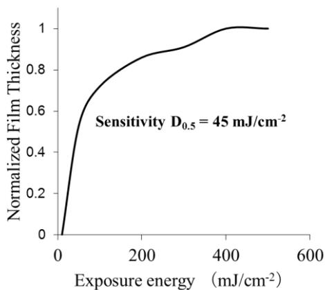
Figure 3. Photosensitivity curve
