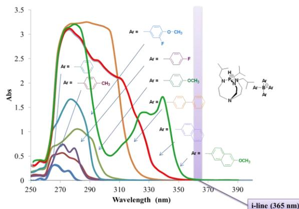
Figure 1. UV-vis spectra of PBGs ( $1.0 \times 10^{-4}\text{M}$ ) in DMAc.
