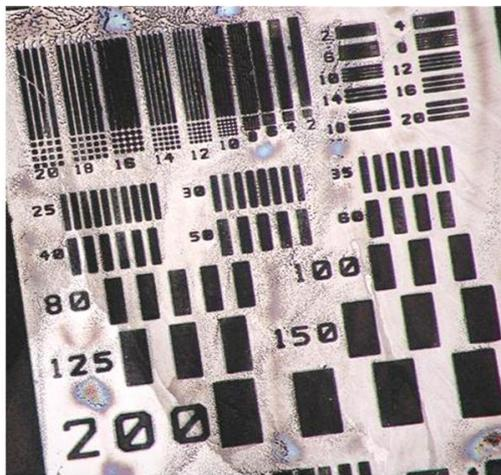
Figure 4. Optical micrograph image fabricated from epoxy resin – PMA-PMMA (20:80). The polymer solution in THF was spincoated at 500 rpm for 10 s, prebaked at 80°C for 5 min, irradiated with 365-nm light at 400 mJ/cm<sup>2</sup>, PEB at 180 °C for 15 min, and developed with THF for 10s.
