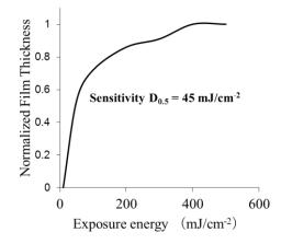
Figure 3. Photosensitivity curve
