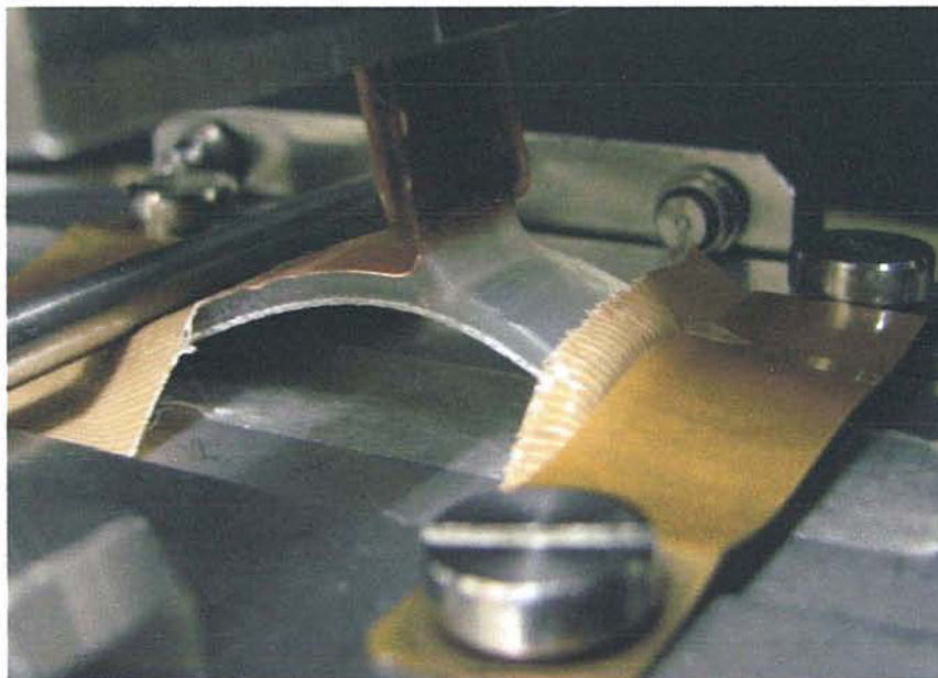
Fig. 4-7. Photographs of peeling test for elastomer plating.
