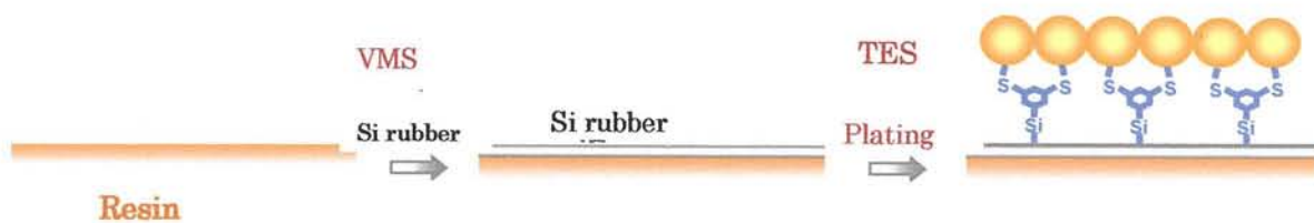
Fig. 4-12. Illustration of plating for improved Q
