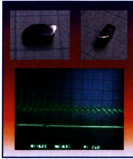
Figure 6.6: The picture of Rh_{17}S_{15} (upper), and pulse echo of this sample (down).
