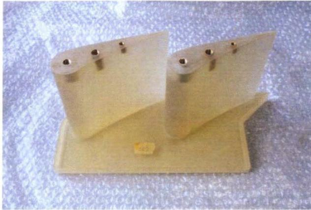
Figure 14 Test blade manufactured by rapid-prototyping method
