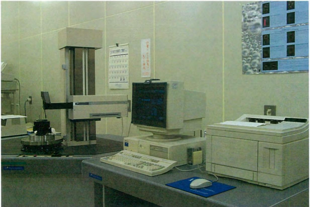
Fig.2.7 Photograph of the roundness measurement equipment
