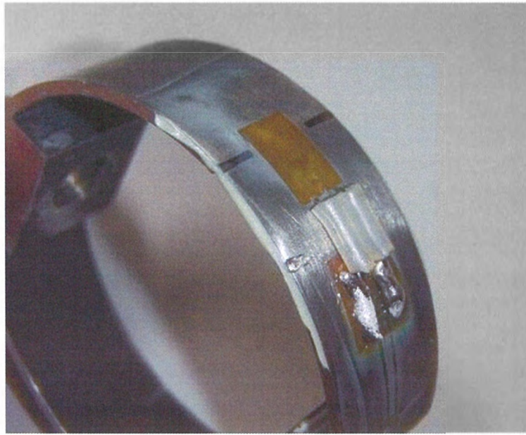
Fig. 2.6 Photograph of the strain ring
