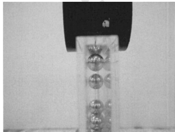
FIG. 3. Side view of a floating iron ball. It floats in between two plastic walls.
