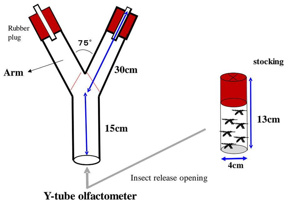
Fig. 3-2. Over view of Y-tube olfactometer to quantify host searching behavior to the odor (i.e. yeast-generated CO<sub>2</sub> and ethyl alcohol).
