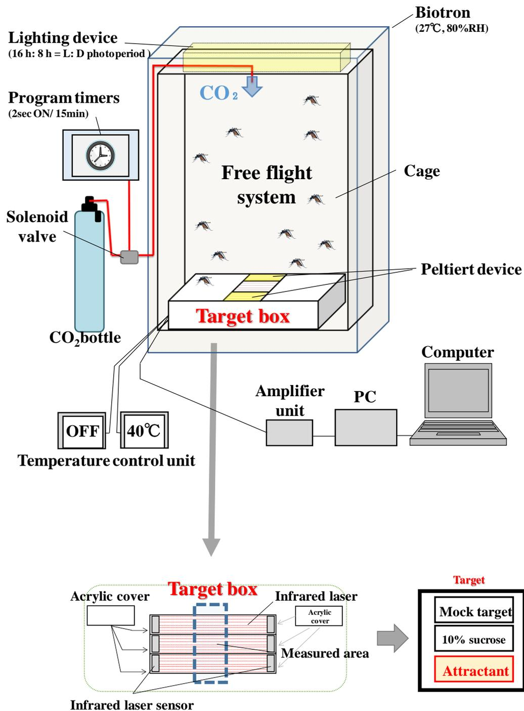
Fig. 3-1. Over view of automatic recording device to quantify host searching behavior to each attractant (see Materials and Methods).
