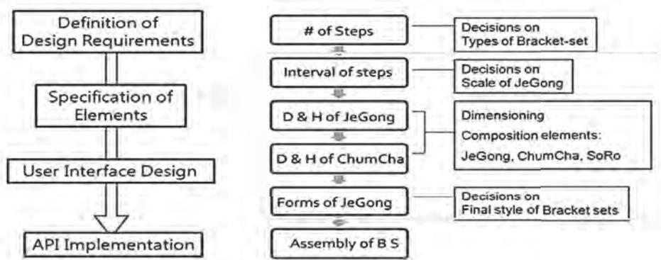
Fig. 4. Implementation of the bracket-set design module
