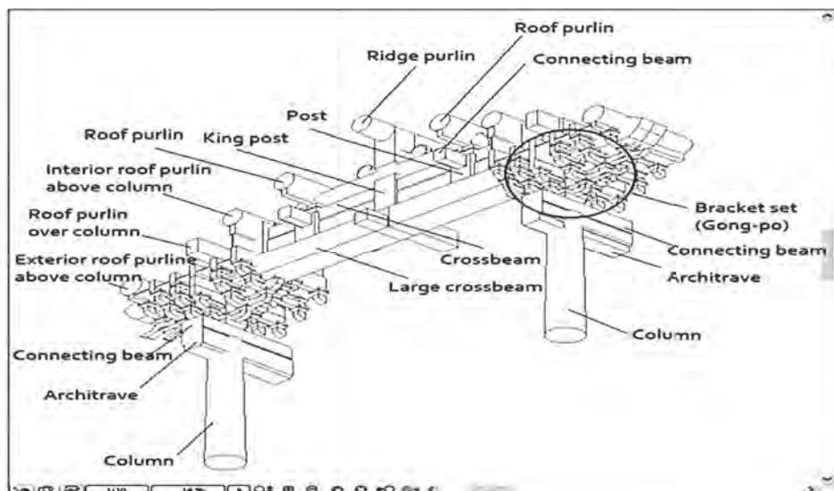
Fig. 2. Element naming surrounding bracket set structure
