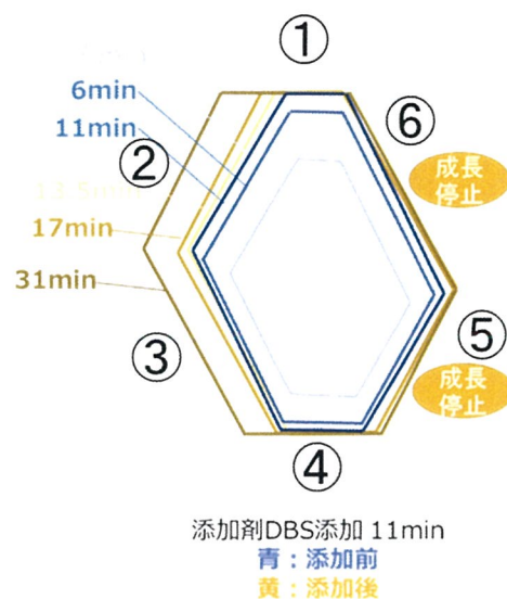
Figure 4-4. Outlines of the crystal before and after addition of DBS. Outlines of the crystal taken at the time shown in the figure was superimposed. (Blue line) outlines of the crystal before addition of DBS, (Yellow line) outlines of the crystal after addition of DBS.
