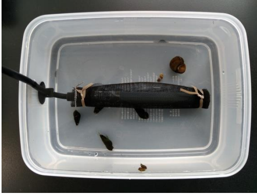
Fig. 3.4 The heater immersed inside the plastic container used in community level experiment.
