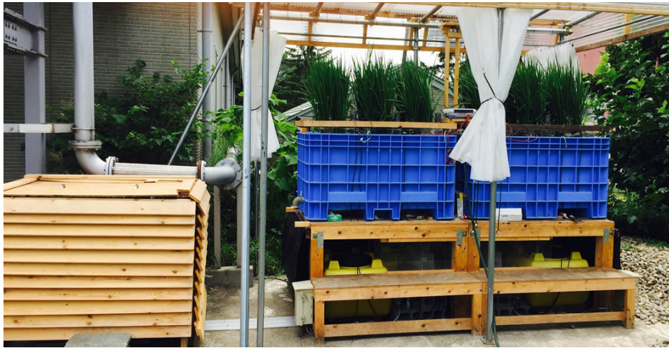
Figure 1.2. Bench-scale experiment to reveal the performance of TWW irrigation to cultivate rice for animal feeding.
