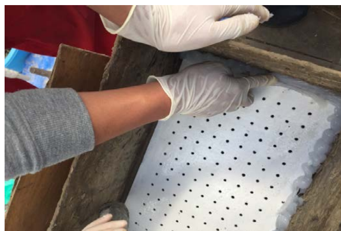
Fig.11 Iron plate on polluted soil
