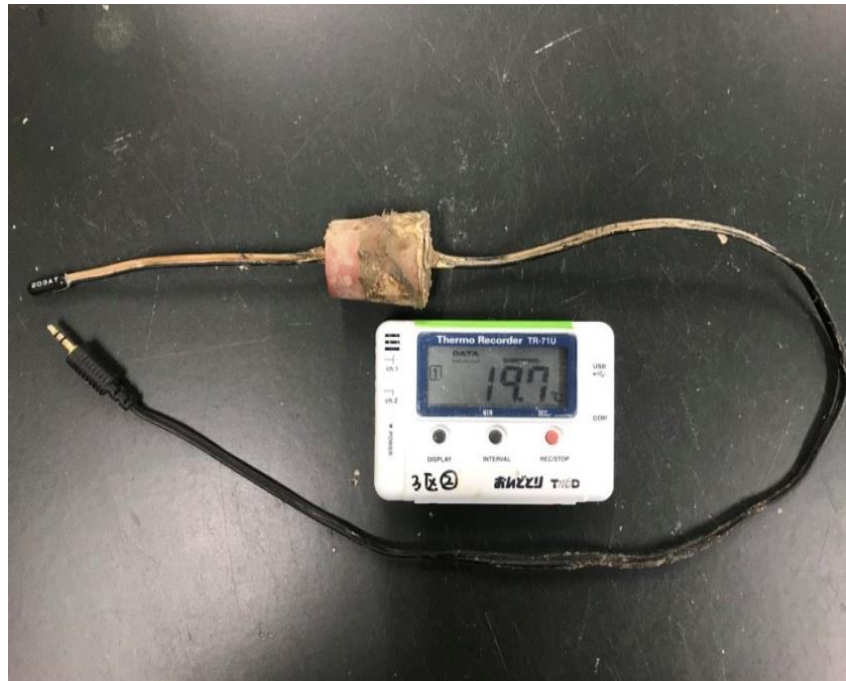
Fig. 29 Temperature sensor and Thermo Recorder TR-71U
