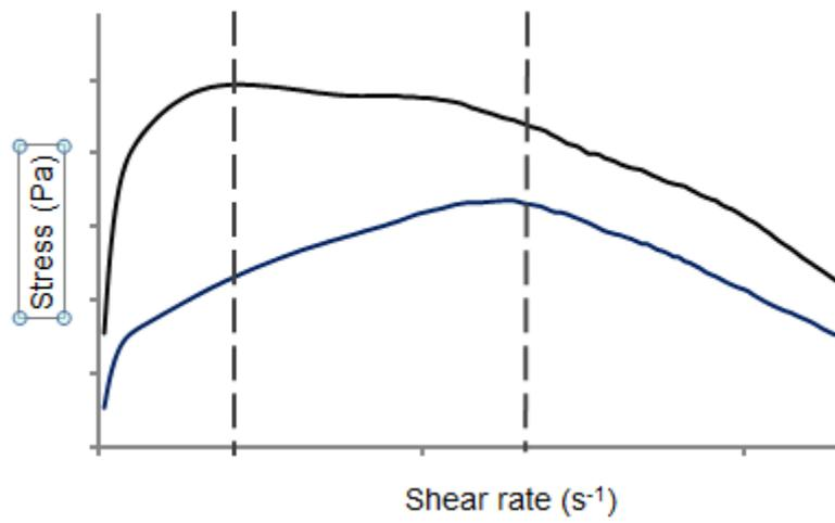
Figure 6. Representative curves showing shear-thinning after the yield point (black) and shear-thickening with a slight increase in shear rate after the yield point before the onset of shear-thinning (blue).
