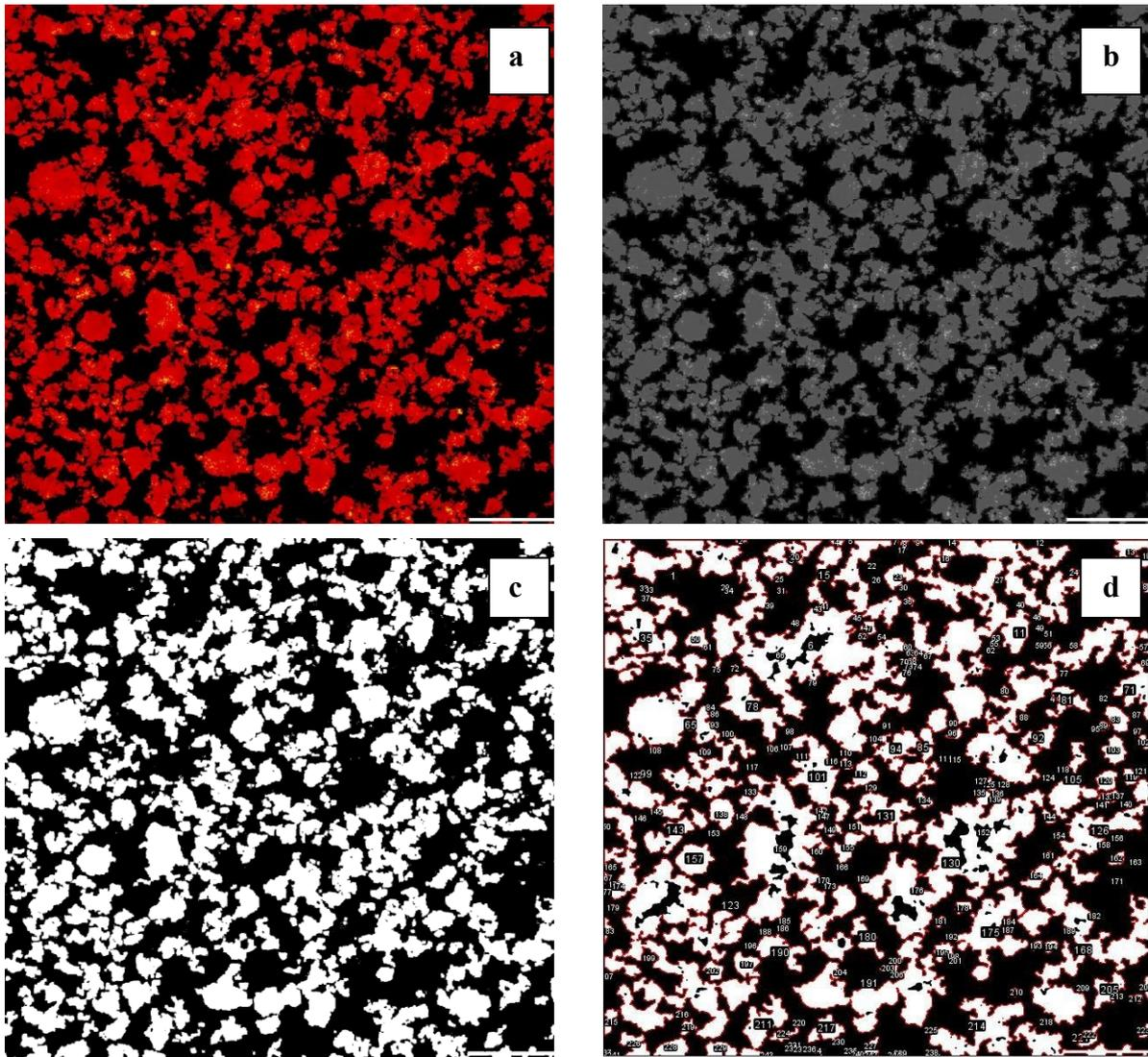
Figure 13. Representative two-dimensional images of TSA-1 yoghurt showing the image analysis process (a) original image, (b) grayscale image, (c) binary image and (d) segmented image for area fraction calculation.
