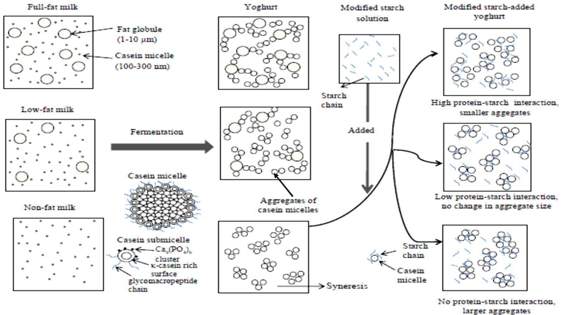
Figure 2. A schematic representation of the formation of stirred yoghurt gels from pasteurized milk to stirred yoghurt followed by the addition of modified starches
