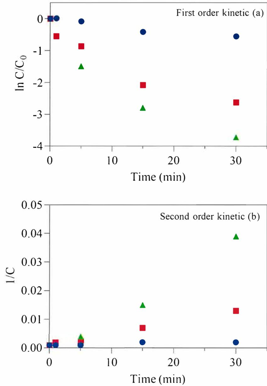
Figure 3.2 Variations of  $\ln (C/C_0)$  (a) and  $1/C$  (b) in water samples over time with different Fe(VI) dosages. Experimental condition: NP = 1 mg/L, initial pH = 6.
