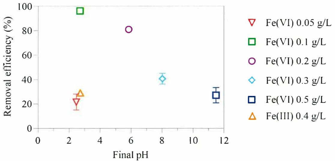
Figure 3.14 Relation between final pH and NP1EO removal efficiency from sludge samples with different Fe(VI) dosages.
