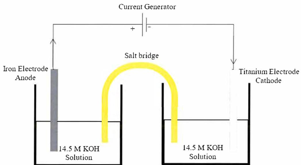
Figure 2.2 Schematic diagram for the electrochemical synthesis of ferrate(VI).
