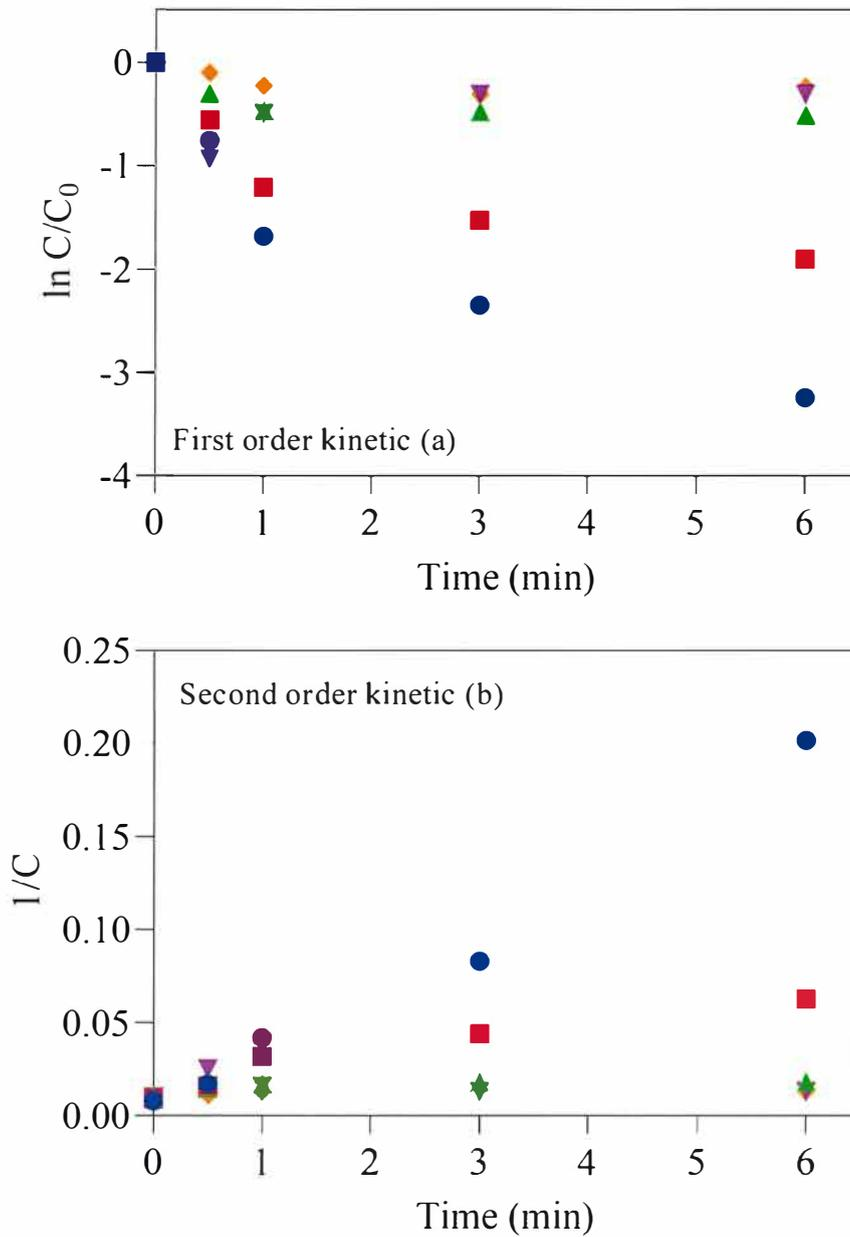
Figure 3.13 Variations of  $\ln (C/C_0)$  (a) and  $1/C$  (b) over time for sludge samples with different Fe(VI) dosages. Experimental condition: NP1EO = 100  $\mu\text{g/L}$ , initial pH = 2.
