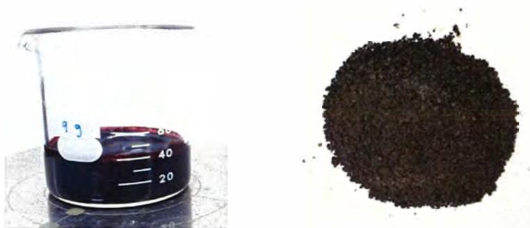
Figure 2.1 Mixing of chemicals (left) and powdered precipitate of  $K_2FeO_4$  after freeze-drying (right).
