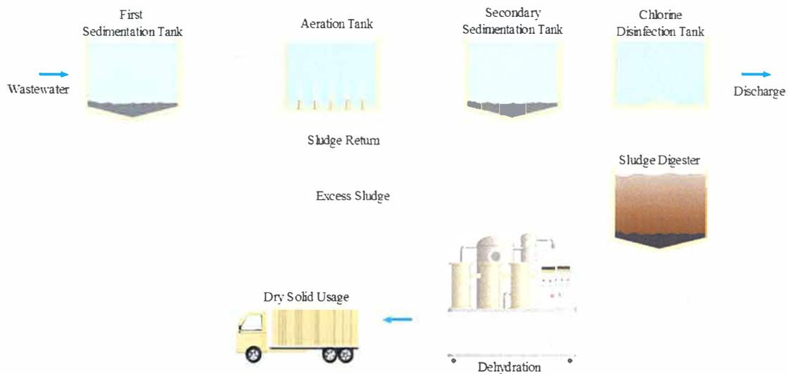
Figure 1.1 Schematic diagram of wastewater treatment processes.
