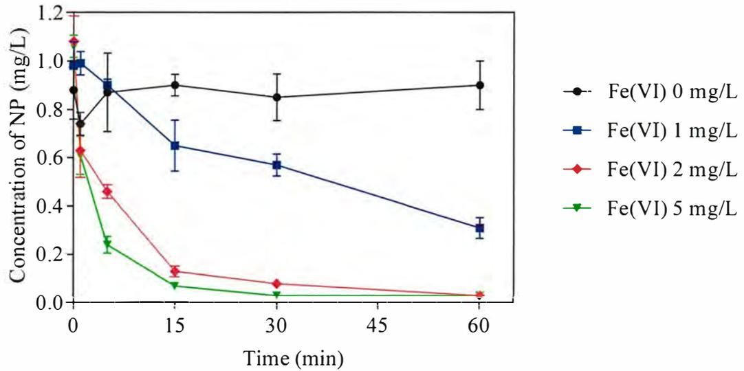
Figure 3.1 Variation in NP concentrations in water samples over time with different Fe(VI) dosages.
