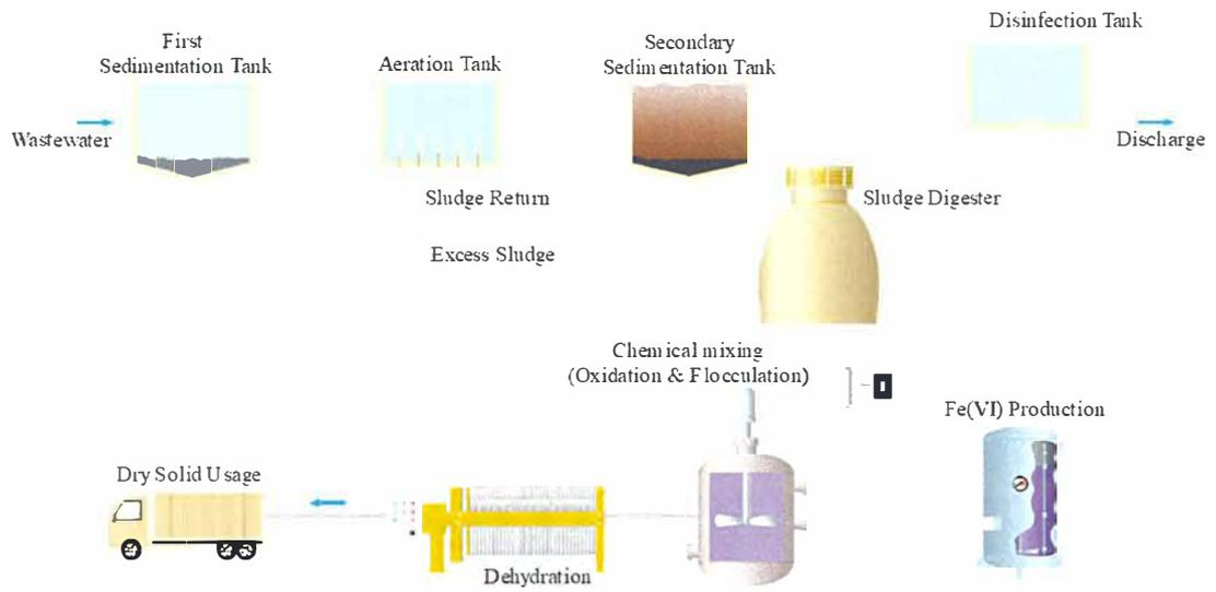
Figure 6.4 Schematic of the possible Fe(VI) oxidation in the sludge treatment process.
