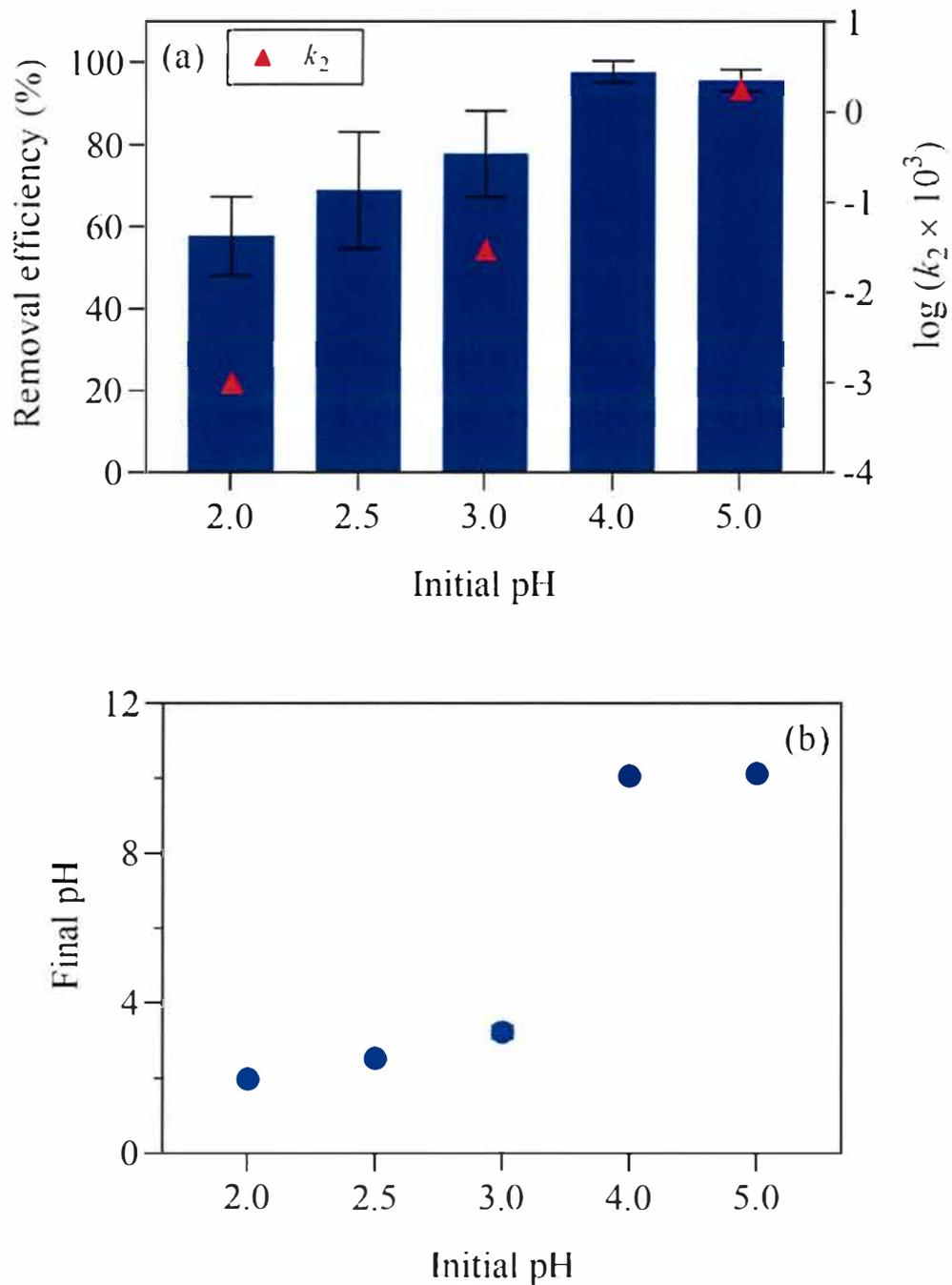
Figure 3.5 NP removal efficiency after 1 h and second order rate constants ( $k_2$ , L/ $\mu$ g/min) (a), and final pH (b) in water samples with a Fe(VI) dosage of 5 mg/L at different initial pH values.
