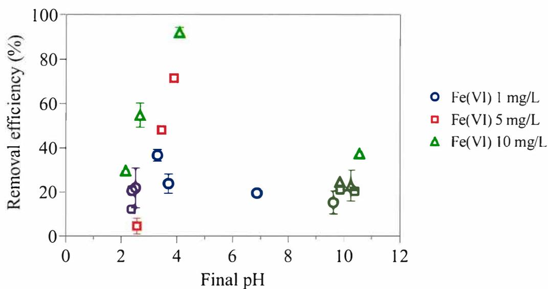
Figure 3.10 Relation between NP1EO removal efficiency and final pH from water samples with different Fe(VI) dosages.
