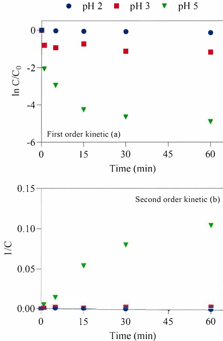
Figure 3.4 Variations of  $\ln (C/C_0)$  (a) and  $1/C$  (b) over time for NP removal by Fe(VI) at different initial pH values. Experimental condition: NP = 1 mg/L, Fe(VI) = 5 mg/L.
