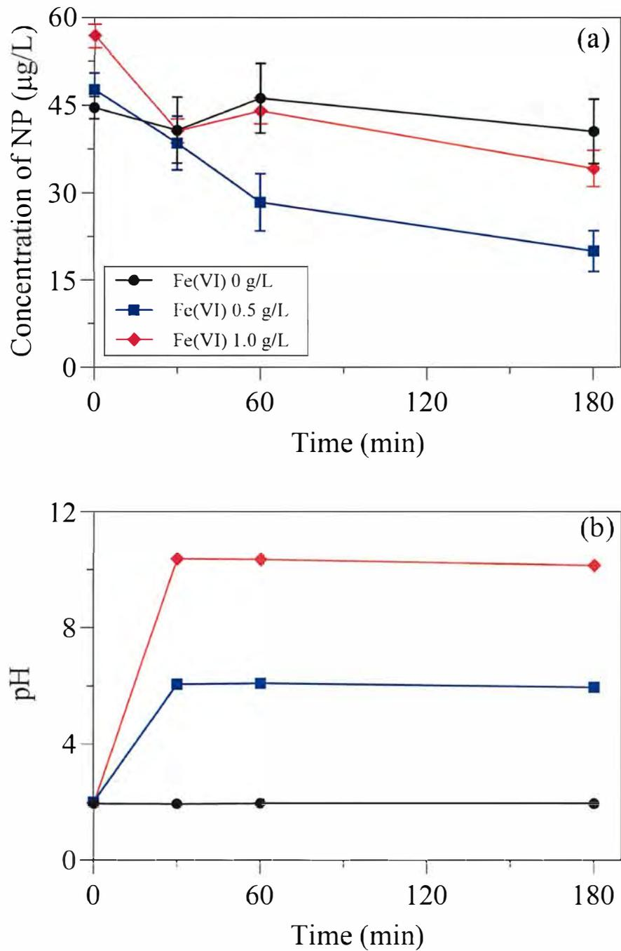
Figure 3.6 Variations in NP concentration (a) and pH (b) in sludge samples over time with different Fe(VI) dosages.
