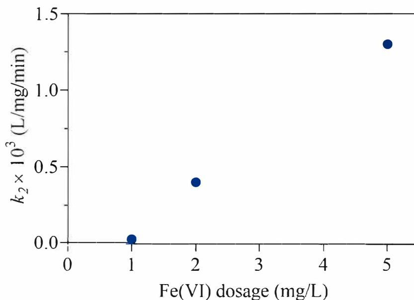
Figure 3.3 Relation between second order rate constant ( $k_2$ ) for NP removal by Fe(VI) and Fe(VI) dosage in water samples at initial pH of 6.
