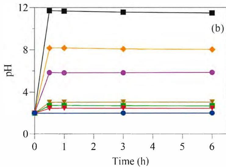
Figure 3.12 Variations of NP1EO concentrations (a) and pH (b) in sludge samples over time with different Fe(VI) dosages.
