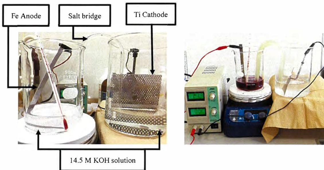
Figure 2.3 Electrochemical synthesis of ferrate(VI).
