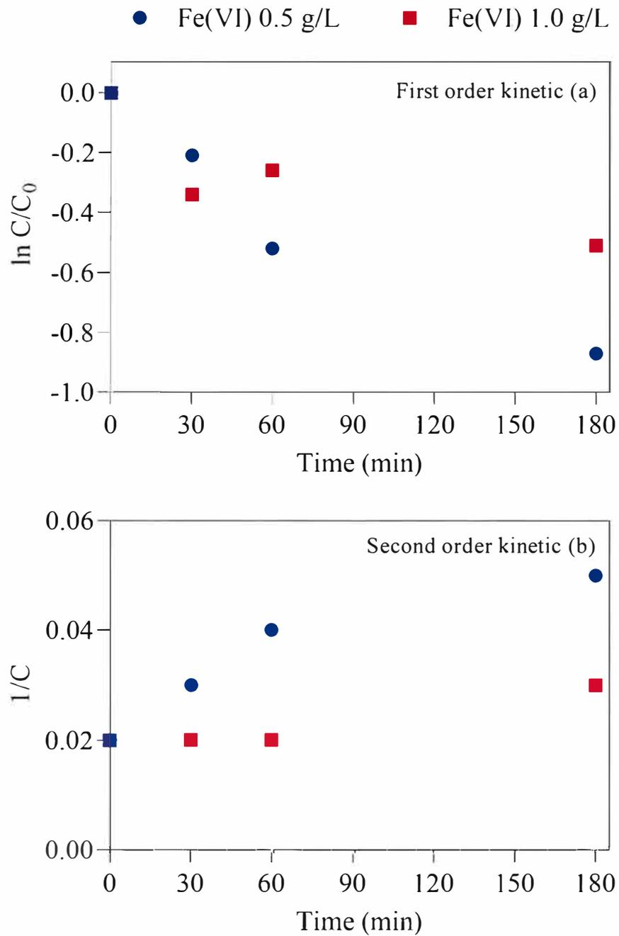
Figure 3.7 Variations of  $\ln(C/C_0)$  (a) and  $1/C$  (b) over time for sludge samples with different Fe(VI) dosages. Experimental condition: NP = 50  $\mu\text{g/L}$ , initial pH = 2.
