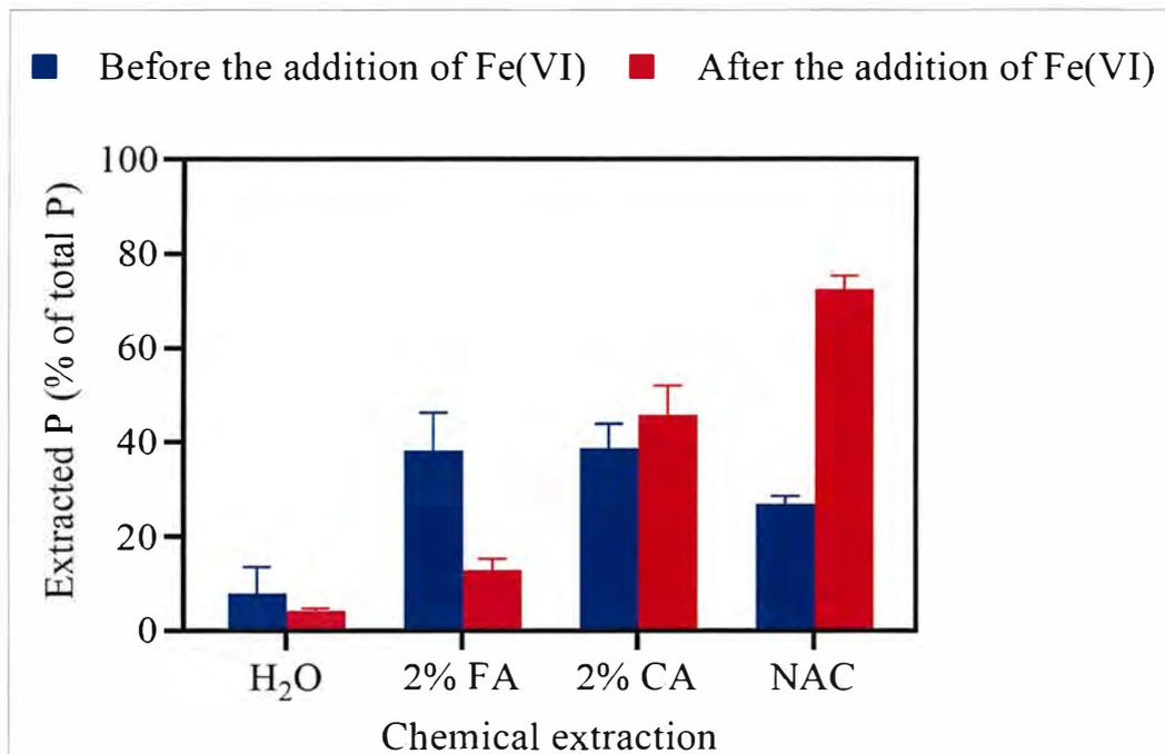
Figure 5.1 Extraction efficiencies of phosphorus from sludge solid phase with H<sub>2</sub>O, 2% CA, 2% FA and NAC before and after Fe(VI) addition.
