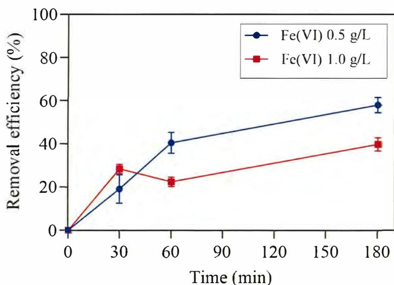
Figure 3.8 Variation in NP removal efficiency from sludge samples over time with different Fe(VI) dosages.
