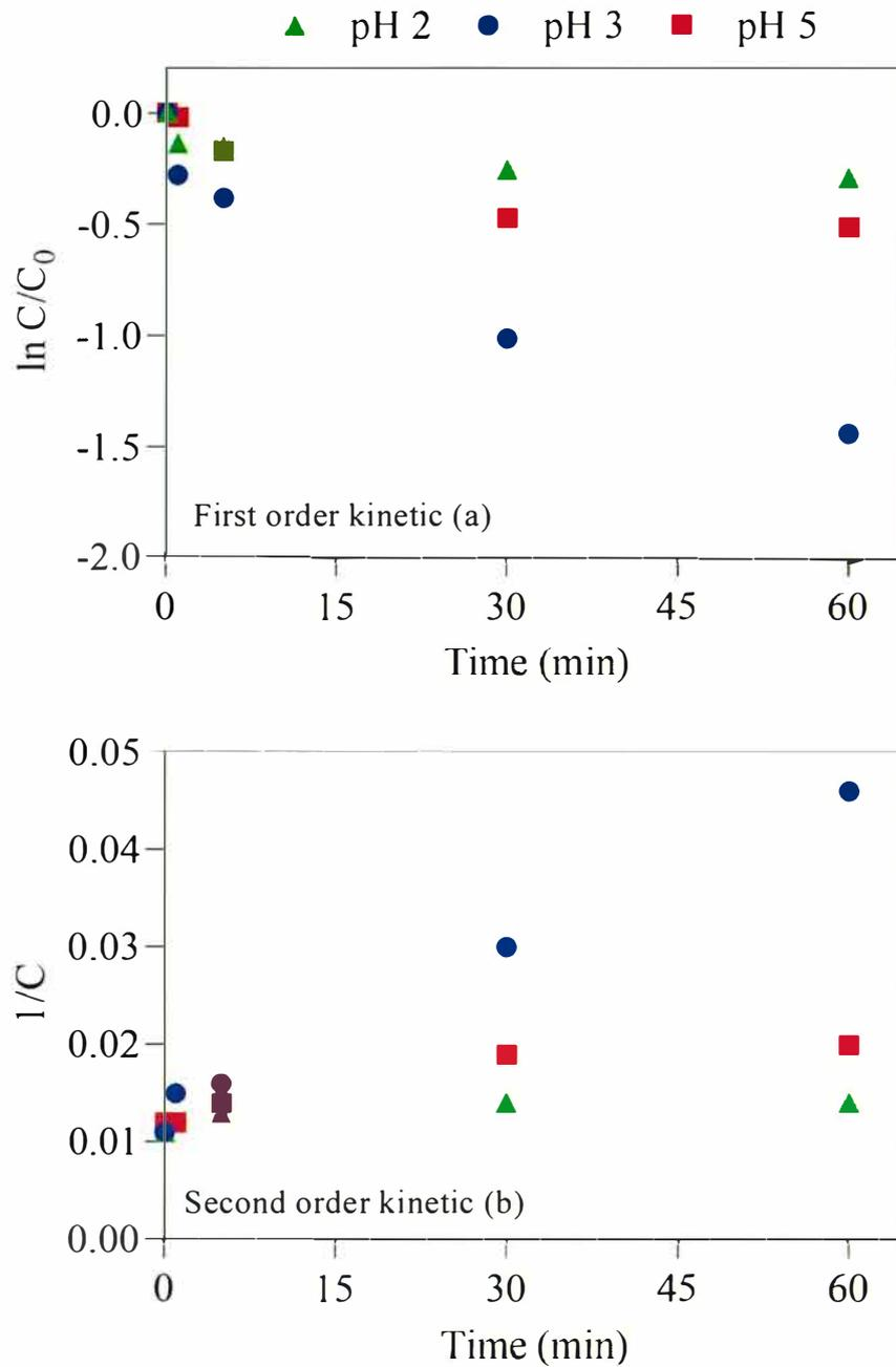
Figure 3.11 Variations of  $\ln (C/C_0)$  (a) and  $1/C$  (b) over time for NP1EO removal by Fe(VI) at different initial pH values.
