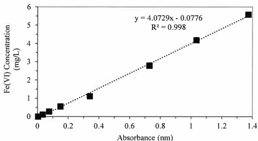
Figure 2.4 Example of calibration curve for the analysis of Fe(VI).
