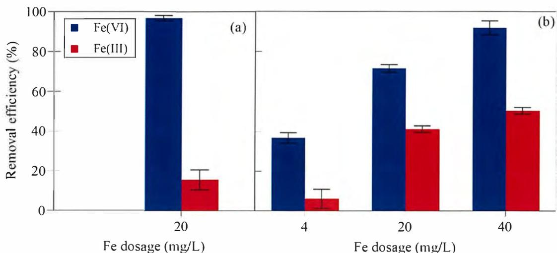
Figure 3.15 Comparison of NP (a) and NP1EO (b) removal between  $K_2FeO_4$  precipitate and  $Fe_2(SO_4)_3$  solution. Experimental condition: initial concentration of NP = 1 mg/L and NP1EO = 100  $\mu\text{g/L}$ .
