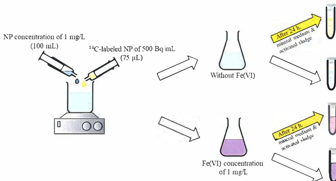
Figure 4.2 Schematic diagram of the experimental procedure for the biodegradability of NP and its degradation products.
