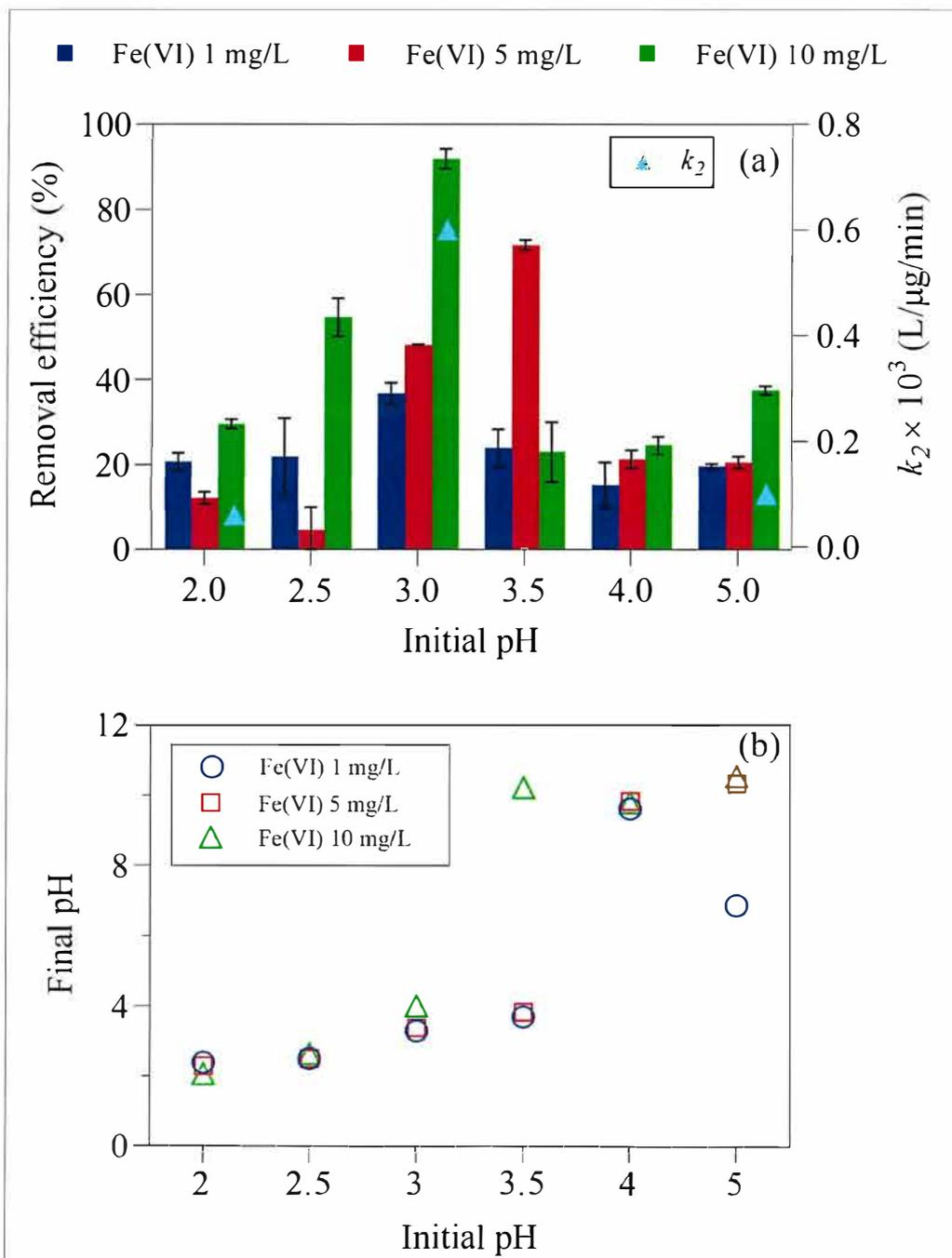
Figure 3.9 NP1EO removal efficiency and second order rate constants ( $k_2$ ) (a), and final pH (b) from water samples with various Fe(VI) dosages and different initial pH values. Experimental condition: NP1EO = 100  $\mu$ g/L. The  $k_2$  values for removal of NP1EO are calculated for a Fe(VI) dosage of 10 mg/L.
