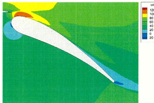
Fig. 3.9: Time-averaged distribution of velocity component u_x by the wall-modelled Navier–Stokes simulation around the flap when \alpha = 5.5^\circ .
