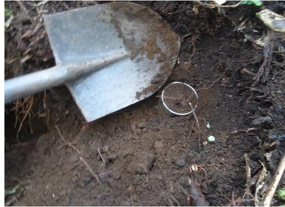
Figure 2.5: Core sampling method
