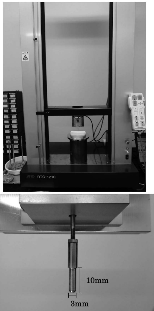
Fig. 2 Micro-indentation test apparatus with double column testing system and indentation rod
