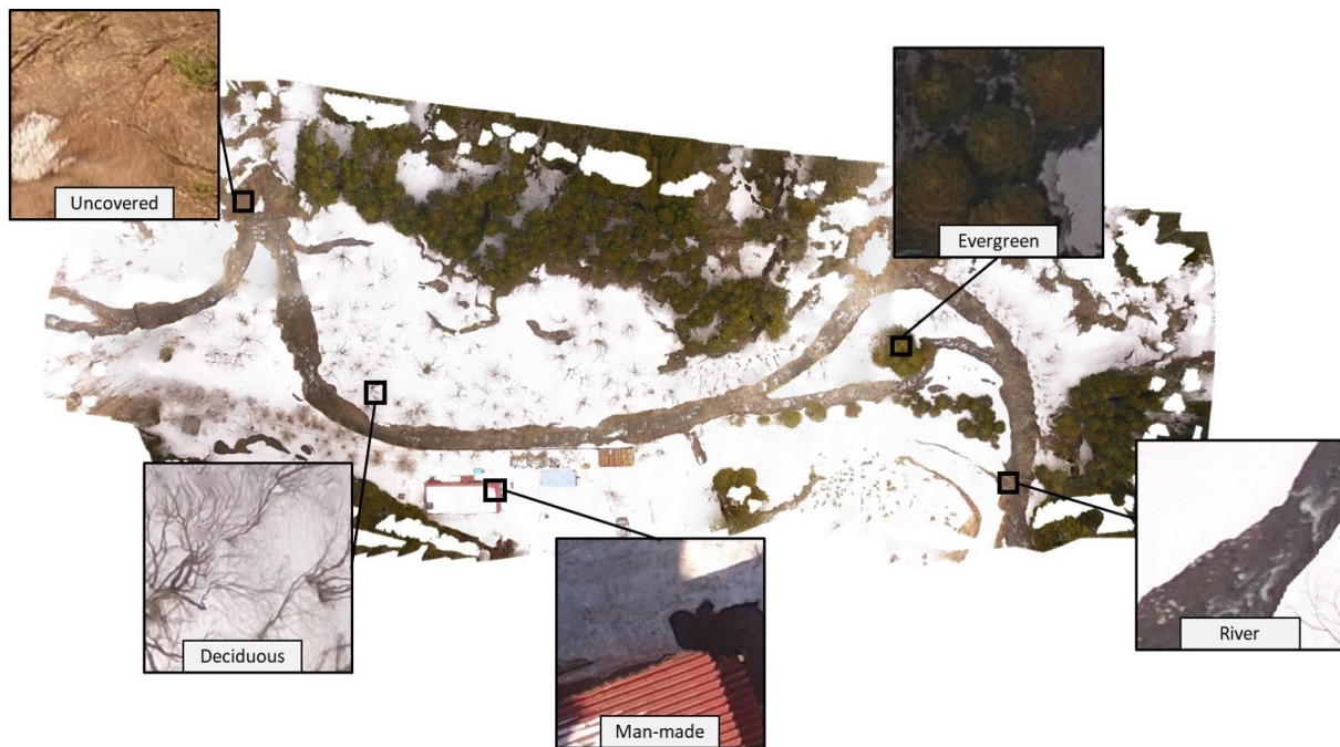
Figure 68 Example of a winter orthomosaic. Examples of patches each containing a single different class
