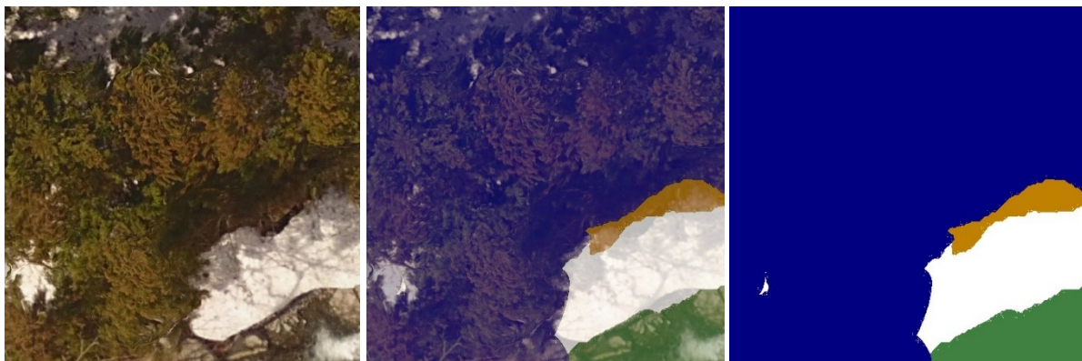
Figure 71 A small section (patch) of a winter orthomosaic. Patch of an RGB Image as captured by the UAV (left). Mask with the annotations showing the class of each pixel (middle), in this case blue pixels belong to the "Evergreen" class, yellow pixels to the "void" class. This mask serves as the ground truth for the semantic segmentation formalisation. Superposition of the two previous images (right). Consequently, the ground truth for this patch was the list [river, uncovered, evergreen] for the multi-label classification formalisation.
