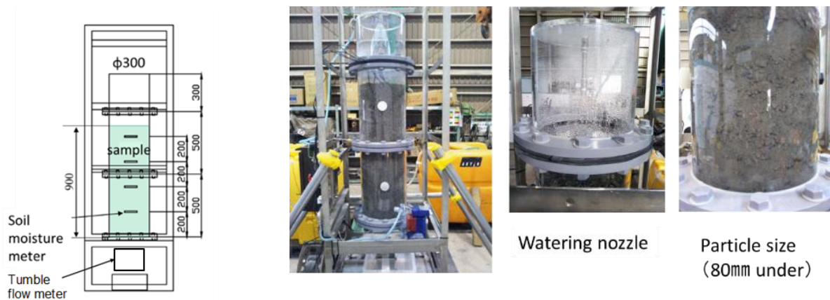
Figure 7.1. Column elution test equipment.
