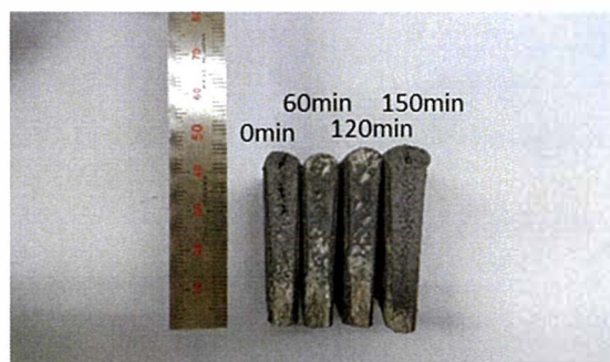
Fig. 5-9 Test piece of chill depth
