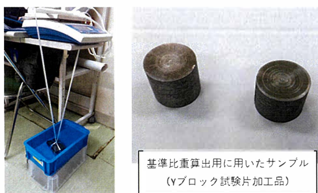
Fig. 5-5 Measurement by the Archimedes method
