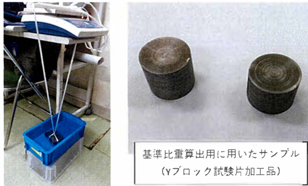
Fig.4-2 Measurement by the Archimedes method
