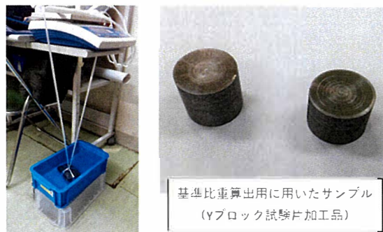
Fig. 2-4 Measurement by the Archimedes method
