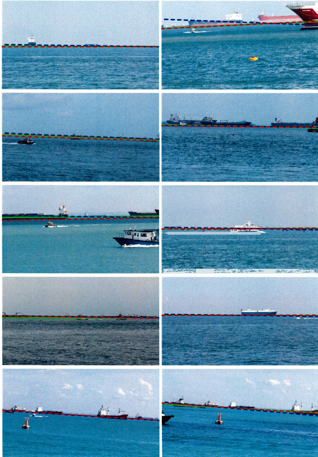
Figure 3.12: Sample frames of detection results the onshore dataset of SMD. (c) Detection results on BD. The red and blue dashed lines indicate the detection result of the horizon line and the coarse-step optimization result, respectively, and the green line indicates the ground truth.
