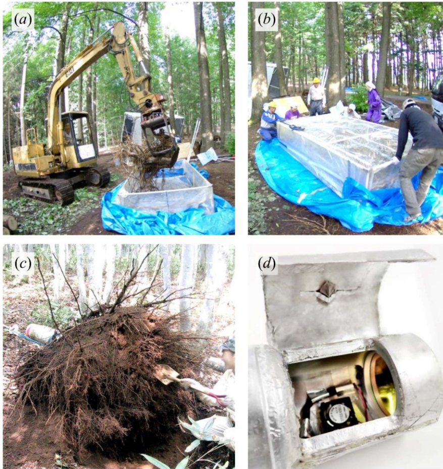
Figure 2.2 Measurement of whole-plant respiration using closed-air circulation chamber. (a) measurement of excavated whole root from a mature tree. (b) Sealing of the material from a mature tree in the chamber. (c) The roots of a mature tree immediately after excavation. (d) Measurement of the germinating seeds, using the smallest chamber ( 80 \text{ cm}^3 ). The seeds are wrapped in a wet sheet and attached to the top cover of the chamber. A small fan is attached to the inside of the sensor head.
