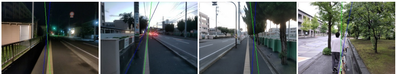
Figure 9. Examples of failure defections. 1st~3rd examples show the case of illumination change and the last example shows the case of obstacles.
