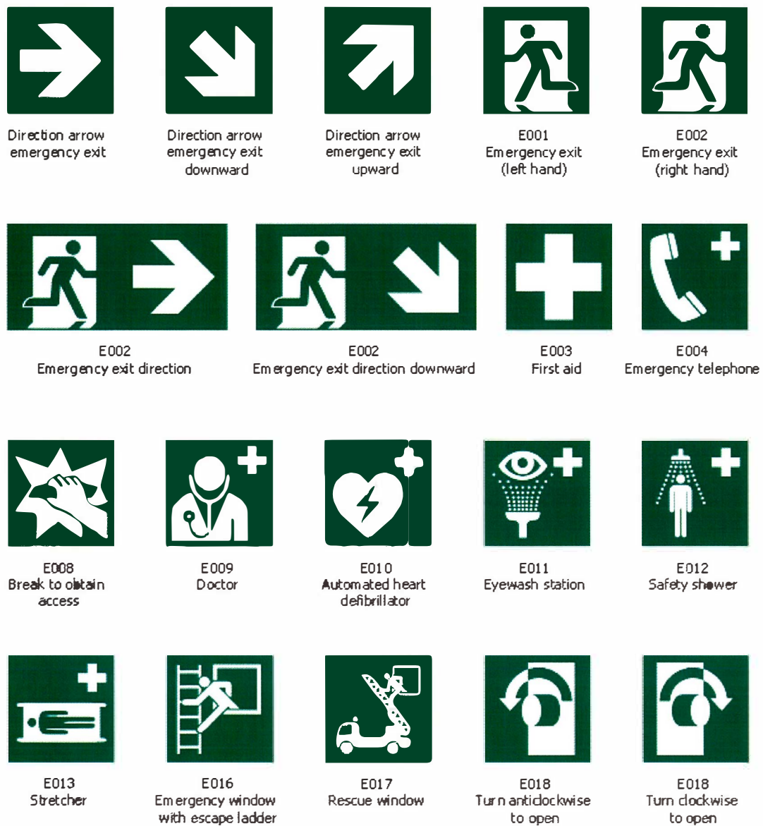
Figure 2.5 International Organization for Standardization, a technical standard for graphical hazard symbols
