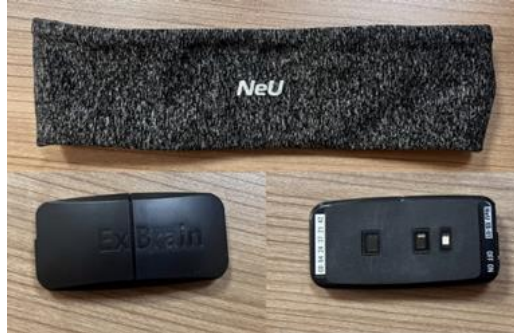
Figure 29: XB-01 brain sensor in a headband. A sensor must be placed in the upper area of the left eye.
