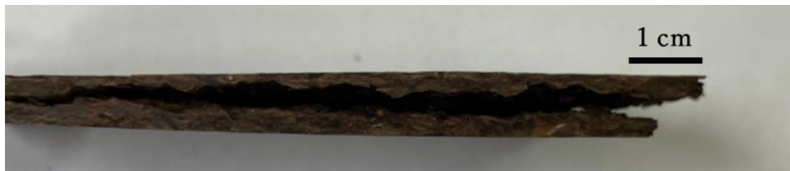
Figure 5-3 The side-view of the board with an internal crack
