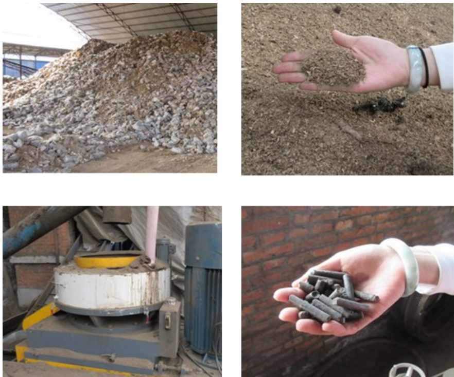
Figure 1-1 Pellet fuel production process from wood ear WMBs
