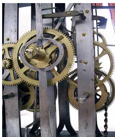
Fig. 25 資料館大時計のムーブメント(前面), 1900年頃, Front view of the movement of the Hall Clock of Iwate Univ., circa 1900 (October, 2006)
