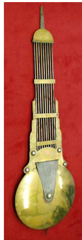
Fig. 13 資料館大時計グリデIRON振り子, 真鍮4本, 鋼鉄5本で構成 Gridiron pendulum of the Hall Clock of Iwate Univ. has a set of nine alternating brass and steel rods (4 brass, 5 steel). (October, 2006)
