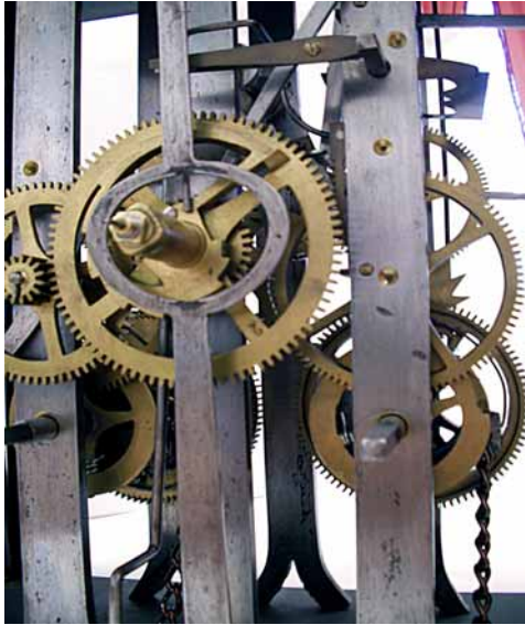
Fig. 25 資料館大時計のムーブメント (前面), 重いグリディロン振り子が付く 1900年頃, Front view of the movement of the Hall Clock of Iwate Univ., Heavy gridiron pendulum is attached. circa 1900 (October, 2006)
