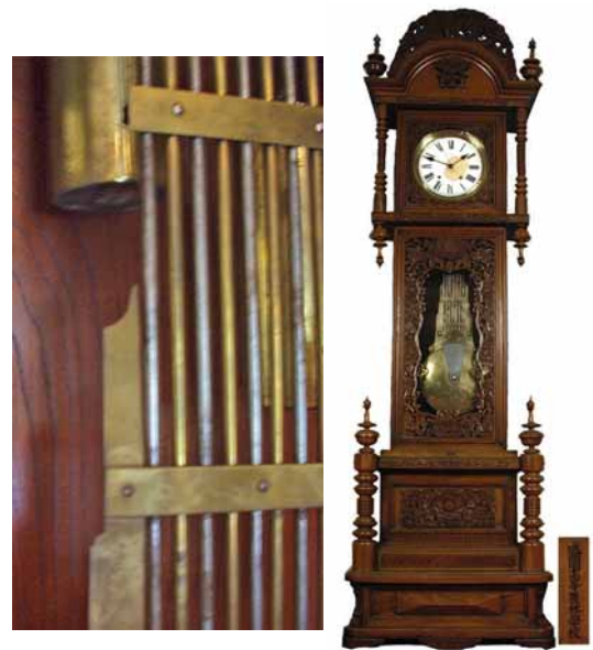
Fig.10 資料館大時計グリデIRON(すの子型)振り子, 9本の棒(真鍮4, 鋼鉄5)で構成 Gridiron pendulum of the Hall Clock of Iwate Univ. has a set of 9 alternating brass and steel rods (4 brass, 5 steel). (June, 2006)
