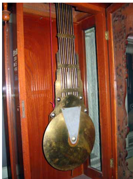
Fig. 18 資料館大時計の大きな温度補償(グリデIRON)振り子, 直径 30cm 円盤付, Heavy, Gridiron (temperature compensation) pendulum with large polished brass disc (30 cm) of the Hall Clock of Iwate Univ. (October, 2006)
