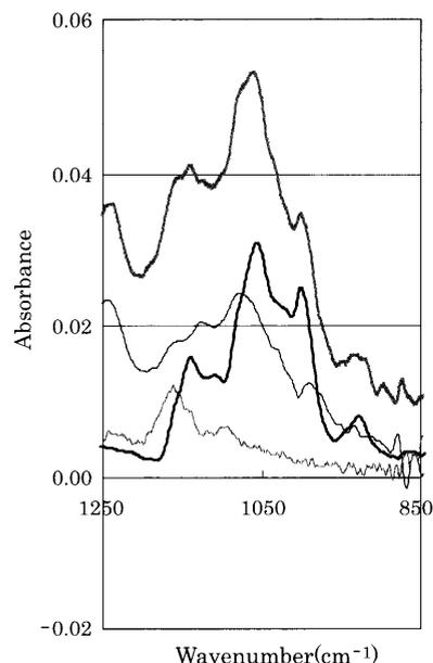
**Fig. 6.** IR spectra of soymilk and its components in C-C and C-O stretching band regions between  $1200$  and  $900\text{ cm}^{-1}$ . Bold gray line, soymilk; bold black line, soy-sugar; simple black line, soy-protein; simple gray line, soy-lipid. The absorbencies of C-C and C-O bands from protein were smaller at  $1000\text{ cm}^{-1}$  and from lipid were negligible.
