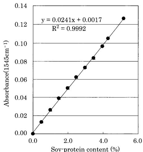
**Fig. 4.** The calibration curve of protein in soymilk. Absorbance of amide II band ( $1545\text{ cm}^{-1}$ ) against soy-protein content is calibrated. Soymilk with changed solid content was used. The protein content of soymilk was determined by the modified method of Bradford. All points have error bars (standard deviation) of data ( $n=3$ ), but the bar was hardly visible because of being so small.
