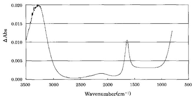
**Fig. 2.** IR spectra of water (using a background spectrum of air).  $\Delta\text{Abs}$  of the vertical axis was obtained by applying IR spectrum of water and the average ratio of absorbance changes by soymilk of 10% solid between 2300 and 1900  $\text{cm}^{-1}$  (that is the small and broad absorption band of water although soymilk components have no absorption).
