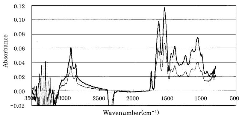
**Fig. 1.** IR spectra of soymilk in various solid contents. IR spectra of soymilk were measured using a FT-IR spectrophotometer equipped with an ATR apparatus. Order of IR spectra from the top is soymilks prepared with 6, 8, 12, and 20 times de-ionized water of the soybean weight.
