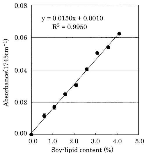
**Fig. 5.** The calibration curve of lipid in soymilk. Absorbance of ester band ( $1745\text{ cm}^{-1}$ ) against soy-lipid content is calibrated. Soy-lipid was prepared as reconstituted oil-body formed by adding soybean oil to defatted soymilk and then treating it ultrasonically. All points have error bars (standard deviation) of data ( $n=3$ ), but they are hardly visible because of being so small.
