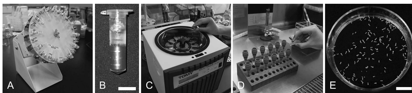
Fig. 1. Improvement of microspore culture for multiple samples. (A) Bud sterilization and washing in 2 ml plastic tubes using a Rotator. (B) A 2-ml plastic tube contained buds and cylindrical metal. (C) Buds were macerated in the tube with cylindrical metal using a Beads Cell Disrupter/Micro Homogenizing System. (D) Microspores were obtained by filtration through a 50 µm CellTrics filter. (E) The improved method produced as many embryos as the conventional method did. Bars (B, E) = 1 cm
