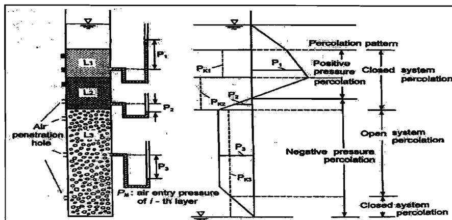
Fig. 2: Pressure head profile and percolation pattern in a stratified soil column (Sasaki, 1995).
