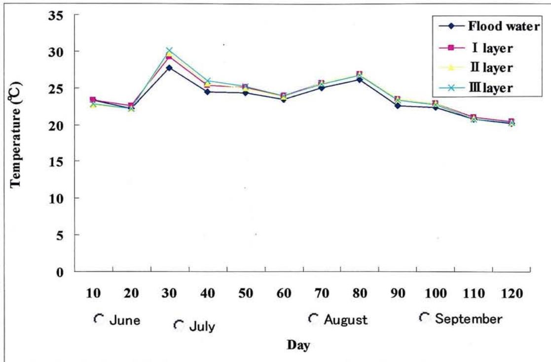
Fig. 33: Temperatures of flood water, plow layer, plowsole and subsoil in open system percolation model: 2009 (M-1 model).
