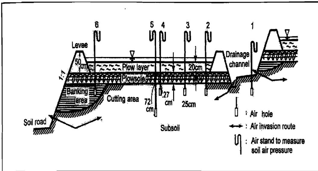
Fig. 1: A schematic diagram of the paddy field used to confirm the occurrence of the open system percolation (Tokunaga and Sasaki, 1990).
