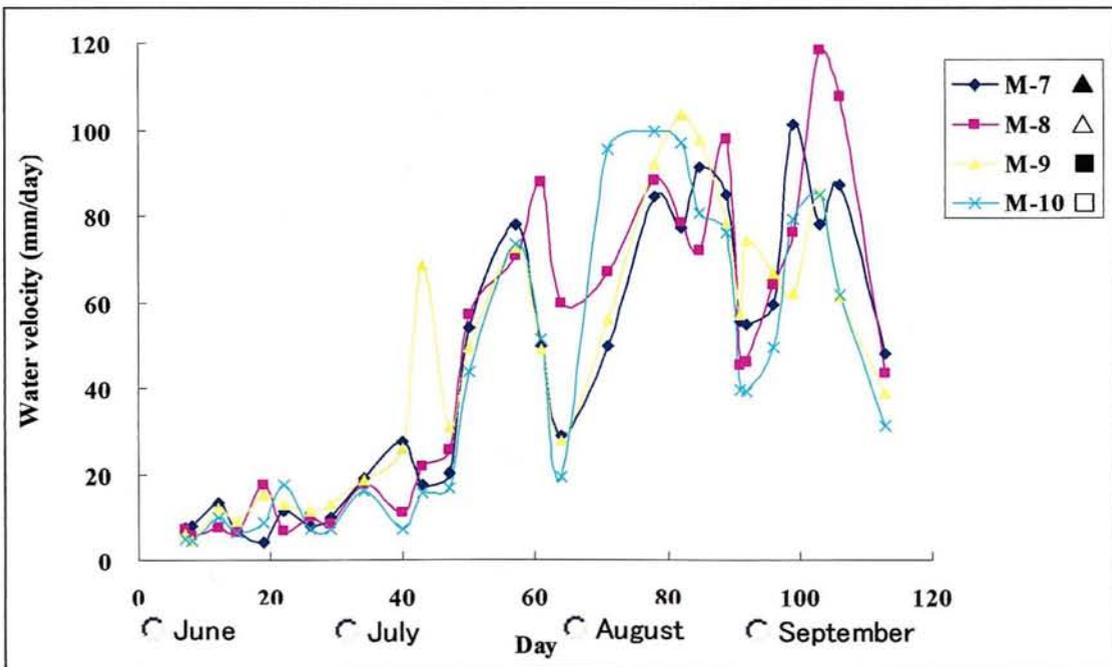
Fig.30: Water requirement rate in stratified paddy field model under open and closed system percolation in 2010 (M-7~M-10).
