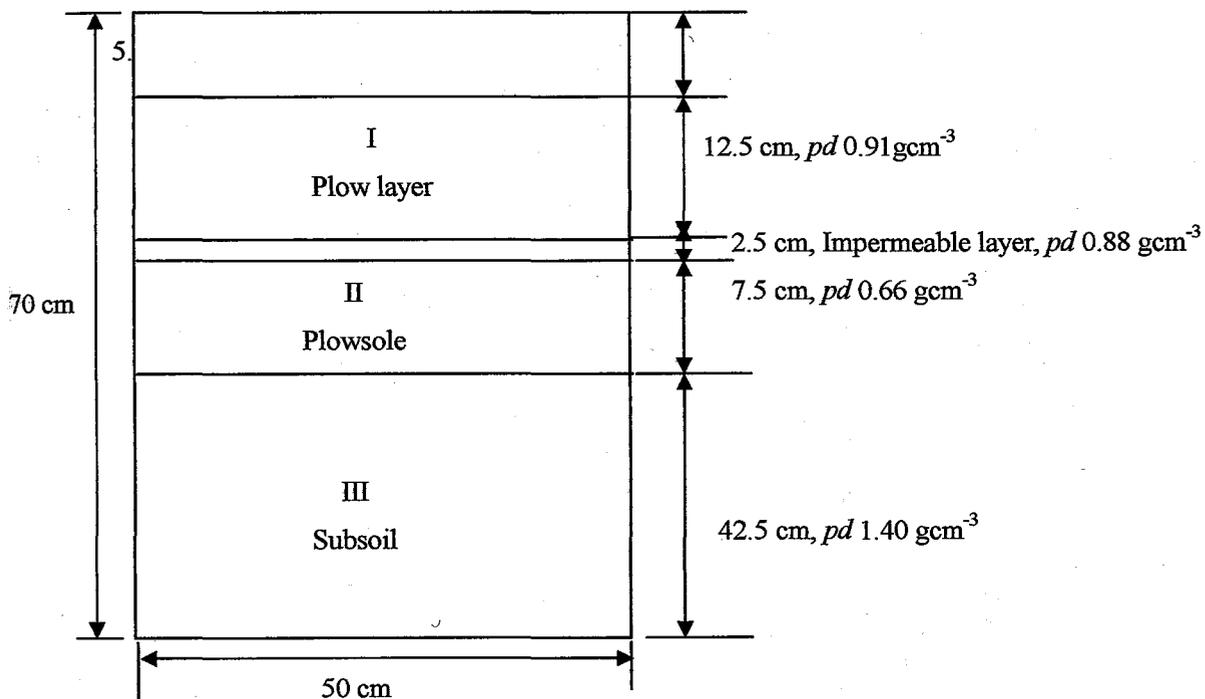
Fig.7: Soil layers of stratified paddy field model.
