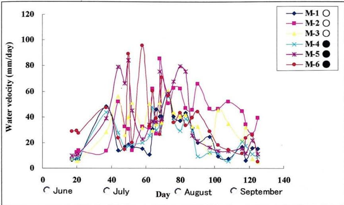
Fig.29: Water requirement rate in stratified paddy field model under open and closed system percolation in 2009 (M-1~M-6).
