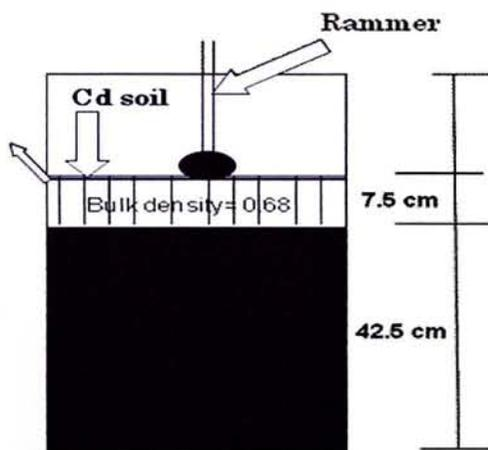
Fig.10 b) Schematic diagram of polluted soil into the iron box.
