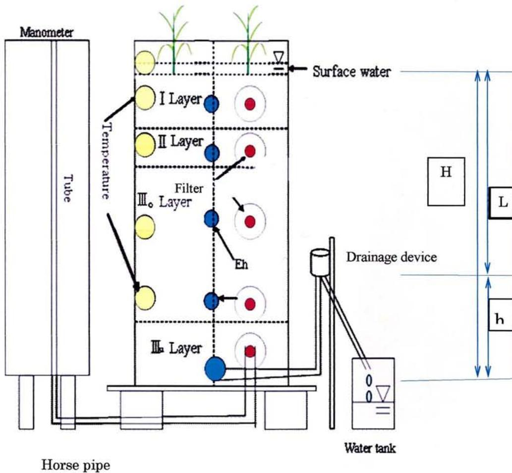
Fig.14: Layout of the experimental device
