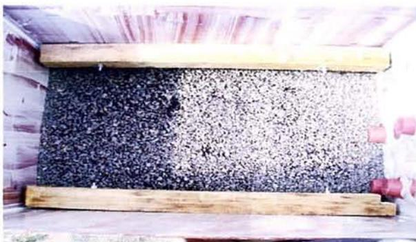
Fig 9: Set up of wood stick in inner side of iron box
