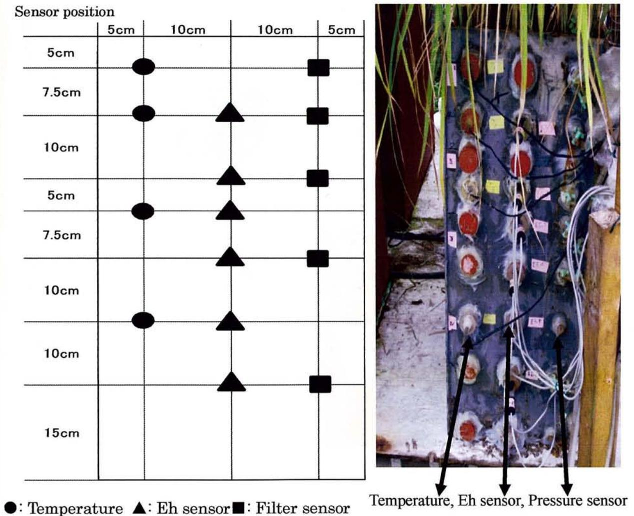
Fig. 15: Sensor position and setting
