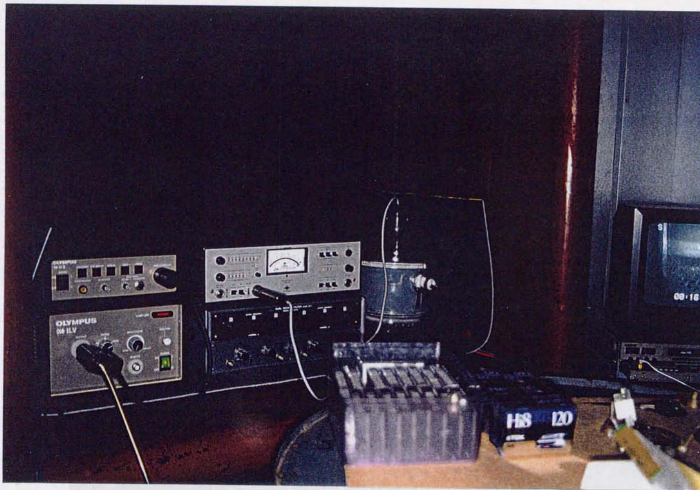
Fig. 14. Sound-recording-equipment arranging from left to right :controller and light-supplier for fiberscope ; amplifier and filter for sound recording ; desiccator chamber with microphone and fiberscope inserted ; monitor and video tape recorder
