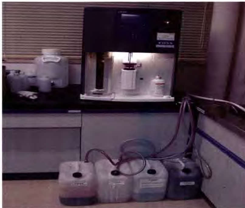
Figure 1.3. Schematic diagram of Foss Kjeltec System (Tecator Digestor System and Kjeltec 2300, Foss Tecator, Sweden) used for determining the N balance
