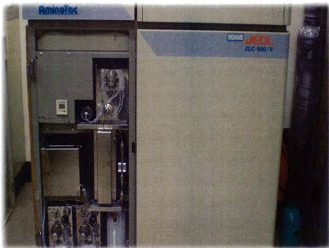
Figure 1.6. Automatic amino acid analyser (JLC-500/V, JEOL, Japan).
