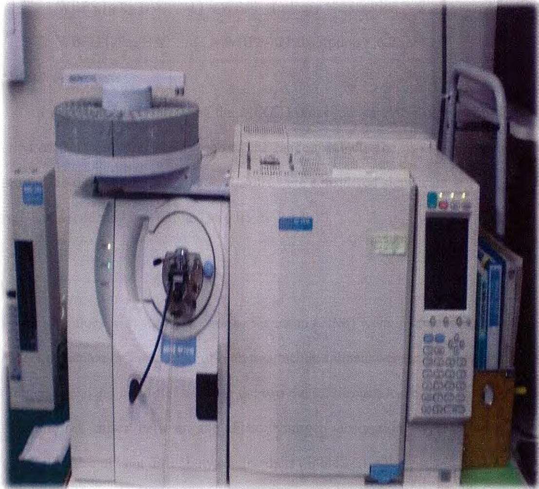
Figure: 1.7. Gas chromatography mass spectrometry (QP-2010, Shimadzu, Japan). Column HP-1, Column temperature 150°C for 6 min, 35°C/min, 300°C for 5 min; Inlet temperature 275°C; Interface and ion mobile phase temperature 250°C.
