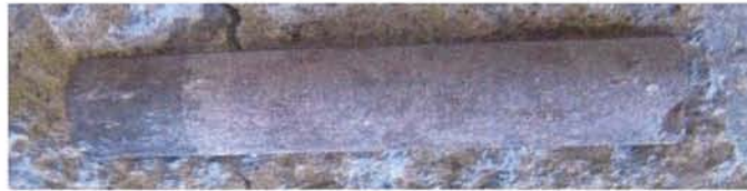
Fig.3-19 Surface appearance of the magnetic corrosion probe B after 70 days corrosion test.
